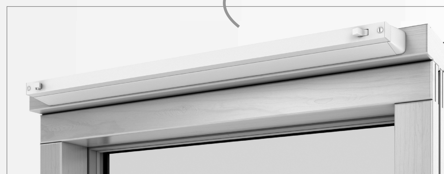
Acoustic trickle vent. The vent is machined into a timber packer with an external aluminium profile in the same colour as the window sashes. Documentation on air flow can be requested. Achieves a sound reduction value of Dn,e,w 40 dB.
